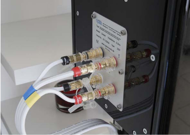
Image 3: Two pairs of heavy-duty WBT terminals mounted on a thick laser carved metal plate taking signals for the High-Midrange iso-dynamic foil transducer and the Mid-Bass woofer separately
